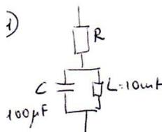
$$\bar{X}_L = 10^{-2} \cdot 100\pi j = \pi \cdot j \Omega = \pi \angle 90^\circ$$
